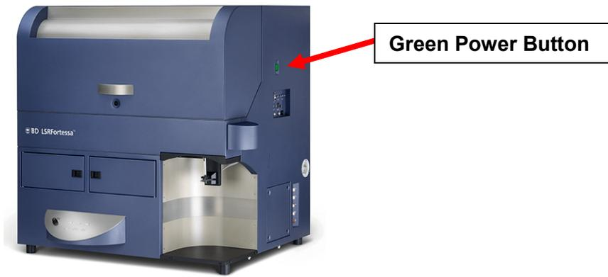
1.4. Ensure that there is a tube with approximately 2 ml of diH<sub>2</sub>O on the SIP. Press the PRIME button to prime the instrument. Repeat priming again after the instrument has returned to STANDBY.
